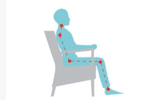
The ideal seat height is obtained when the angle between the upper and lower legs is at least 90 degrees, during which the feet are on the ground.
